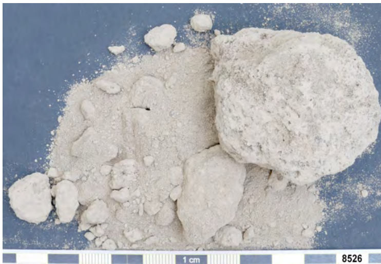
Fig. 13.4 Alchi. Sample 8526. Sample colour (after Munsell): Dry 2.5YR 7/2 light grey. Semi-dry 2.5YR 6/3 light yellowish brown.
