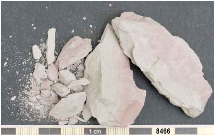
Fig. 6.4 Spituk. Sample 8466. Sample colour (after Munsell): Dry 10YR 7/1 light grey. Semi-dry 10YR 5/2 greyish brown.
