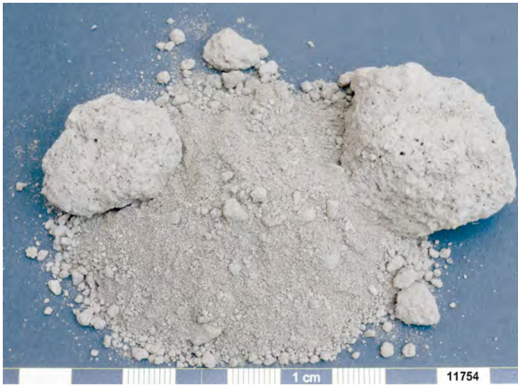
Fig. 8.2 Nyarma. Sample 11754. Sample colour (after Munsell): Dry 5YR 5/2 olive grey. Semi-dry 5YR 3/2 dark olive grey.
