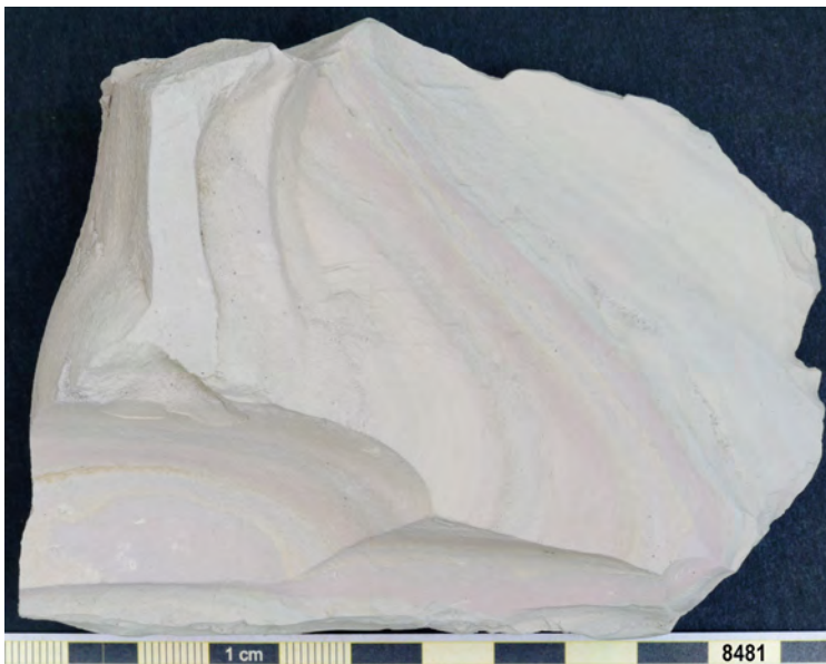
Fig. 7.4 Spituk. Sample 8481. Sample colour (after Munsell): Dry 10YR 6/1 grey. Semi-dry 10YR 4/2–5/2 dark greyish brown to greyish brown.
