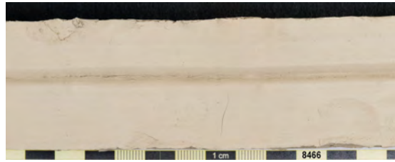
Fig. 10.4 (Top) Sample 8466 from Spituk. Fine surface after the shrinkage test showing just one hair crack.
