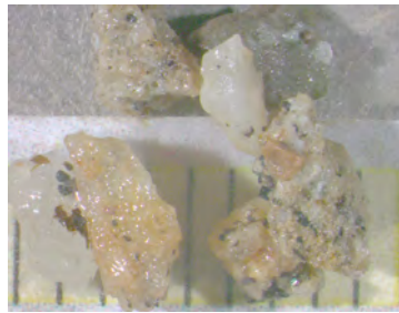
Fig. 33.2 Shapes of grains in sample 8517. Scaled in millimetre. Shape of fraction >2,000 \mu\text{m} (Left and right).
