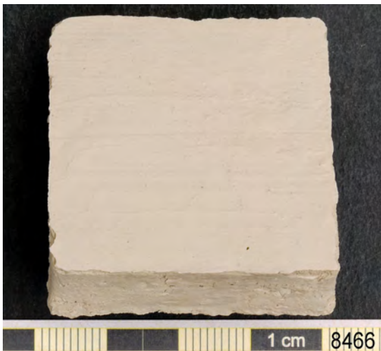
Fig. 12.4 Sample 8466 from Spitik. Specimen used for the hardness test according to Vickers.
