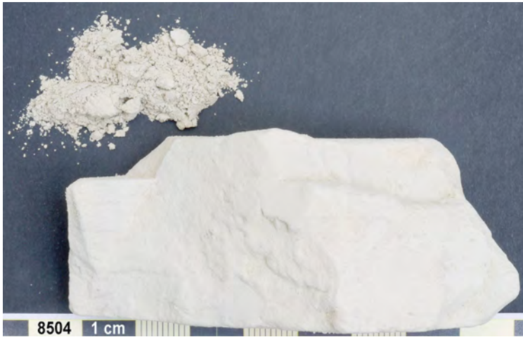
Fig. 34.4 Shelkhar. Sample 8504. Sample colour (after Munsell): Dry 10YR 7/2 light grey. Semi-dry 10YR 6/4 light yellowish brown.
