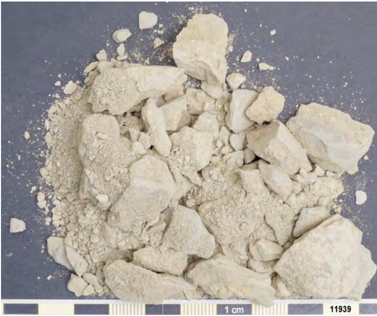
Fig. 19.4 Lamayuru. Sample 11939. Sample colour (after Munsell): Dry 10YR 7/1 light grey. Semi-dry 10YR 6/2 light brownish grey.
