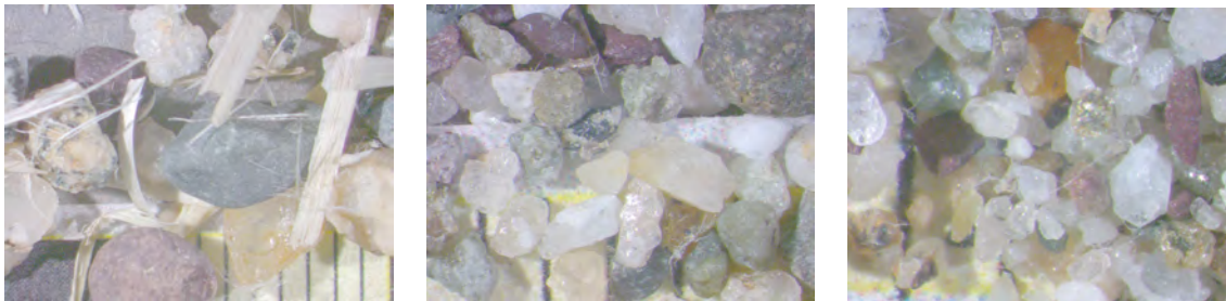
Fig. 56.2 Shapes of grains in sample 11914. Scaled in millimetre. Shape of fraction >2,000 \mu\text{m} (Left), 630\text{--}2,000 \mu\text{m} (Centre), 200\text{--}630 \mu\text{m} (Right).
