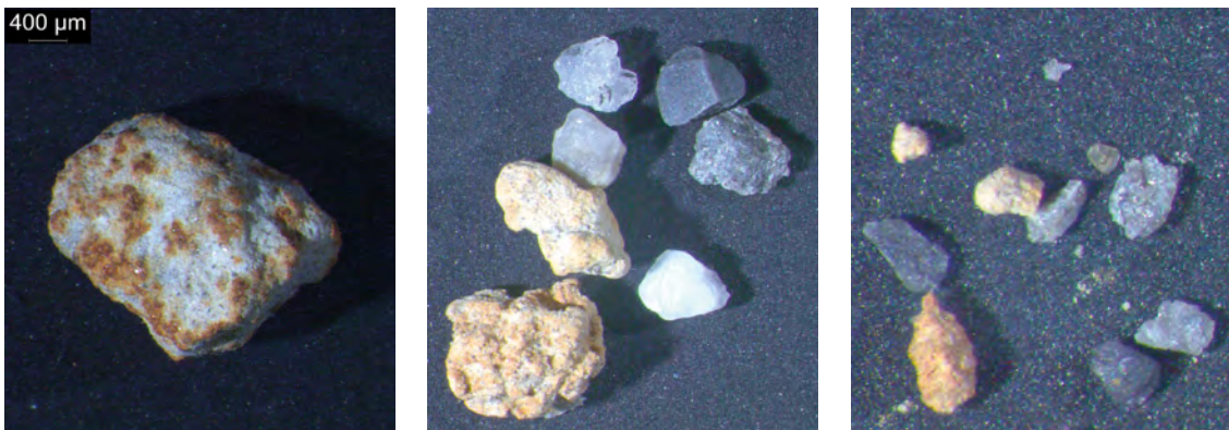
Fig. 5.4 Shapes of grains in sample 6052. Same scale (see upper left corner of the left picture). Shape of fraction >2,000 \mu\text{m} (Left), 630–2,000 \mu\text{m} (Centre), 200–630 \mu\text{m} (Right).
