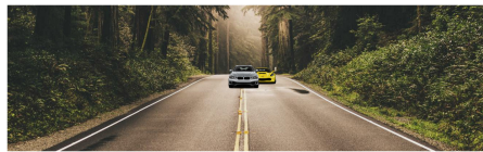
Fig. 4. This image generated by our renderer was misclassified by the NN. The network reported detecting only one car when there were two.
