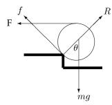
Let the angle between the radius to the point of contact with the step and the downward vertical be  $\theta$ , as shown. At the point of contact, let the frictional force, which is tangent to the sphere, be f and the reaction R (along the radius of the sphere).
