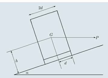
A lorry of weight W stands on a plane inclined at an angle  $\alpha$  to the horizontal. Its wheels are a distance 2d apart, and its centre of gravity G is at a distance h from the plane, and halfway between the sides of the lorry. A horizontal force P acts on the lorry through G, as shown.
