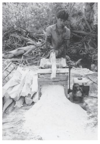
Figure 3.2. Mechanized grinding (mengolah sagu) in an outdoor "sago factory." (Photograph by Wini P. Utari)
