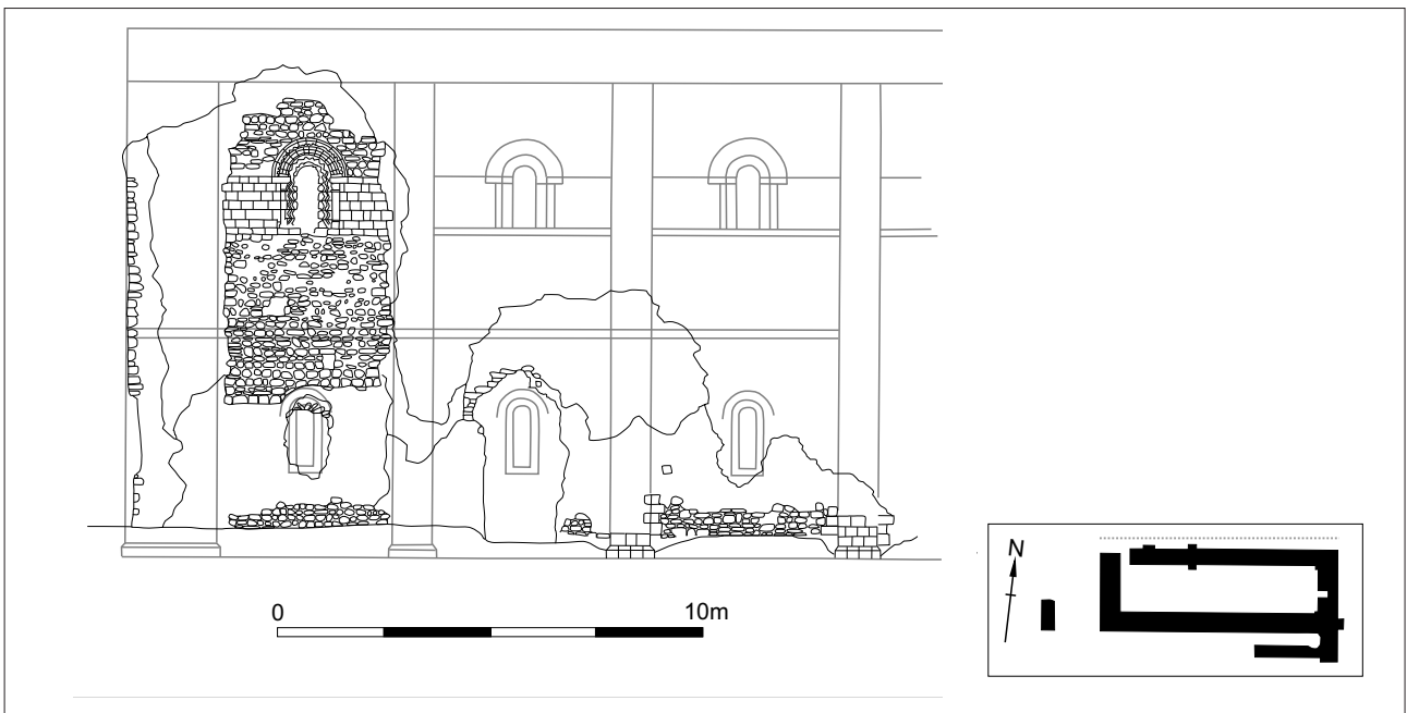
Fig 69 Reconstructed external elevation of the north wall of the north range, c 1135
