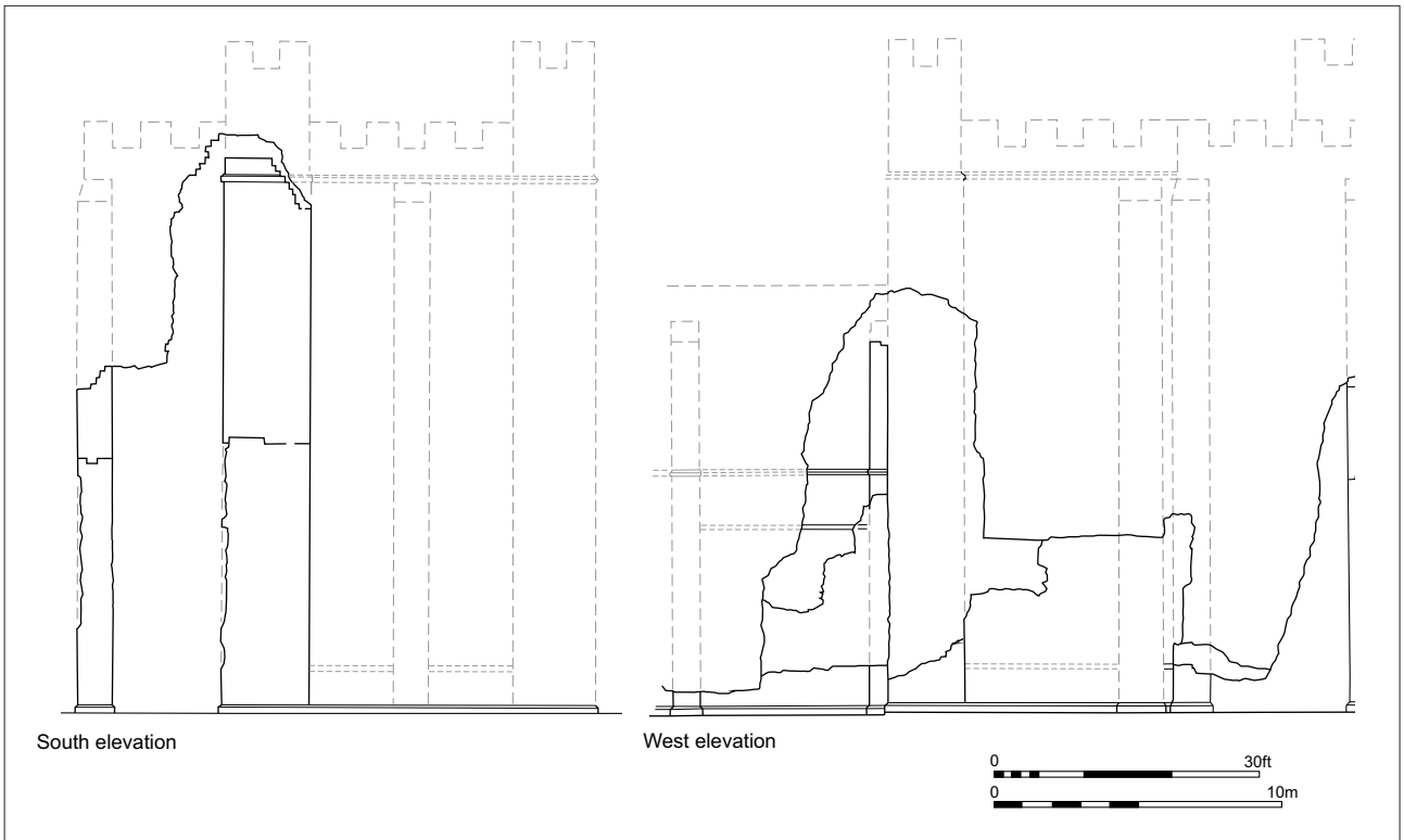
Fig 59 The central building complex: reconstructed south and west elevations of the great tower in Phase I
