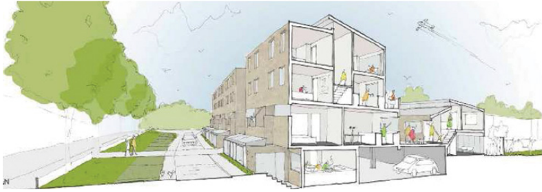
Figure 3.2 Architect’s drawing of Cressingham Gardens’ People’s Plan, showing the additional homes in the garage spaces. Creator of the image: Ashvin De Vos, Variant Office, developed for Cressingham Gardens residents.
