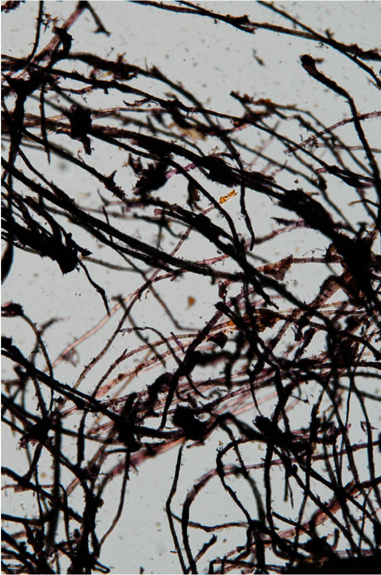
FIGURE 23:9 The long fibres of the Thymeleaceae family plants (possibly Edgeworthia sp.) stained olive-grey with Herzberg in 100×magnification. The book belongs to the British Library Collection, Tib. CC 80.
