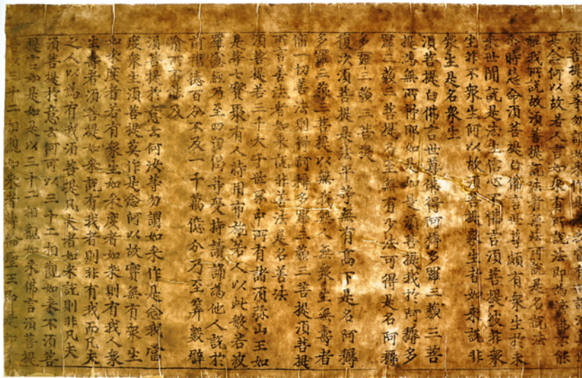
FIGURE 23.3 The paper of the Diamond Sutra's panel 6 viewed against the light. The faint laid lines suggesting the usage of a bamboo sieve attached to the 'floating' mould with a textile sieve visible in this picture. The book is from the British Library Collection.
