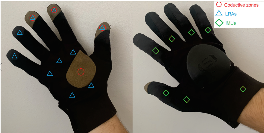
Figure 15.2 Sensors and actuators of Sensorial XR [16].
