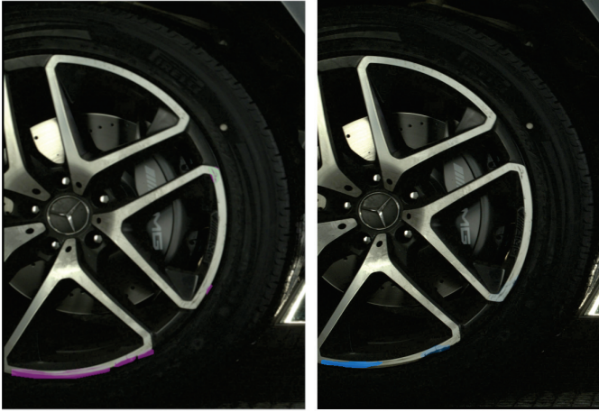
Figure 11.5 Rim damage detection example (target – left; result – right).
