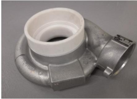
Figure 9. Modular metal casing with cavity insert.
