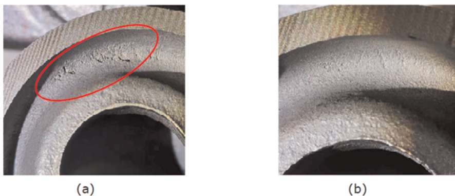
Figure 11. (a) Nitrogen steel with re-oxidation defect (b) Nitrogen steel without defect after optimizing the gating system.
