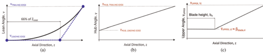
Figure 6. Distribution of (a) lean angle, \nu , (b) tangential angle of the non-radial fibre at the lower end, \gamma_{lower} and (c) tangential angle of the non-radial fibre at the upper end with the leaned straight fibre, \gamma_{upper} , which can be expressed as function of the inlet blade angle, \beta_{blade,4} when z < b_4 .
