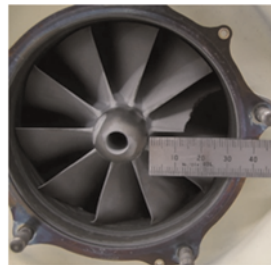
Figure 10: Damaged turbine blade.
