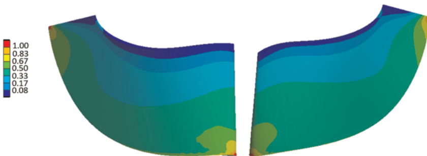
Figure 7. Baseline normalised von-mises stress contour (left – suction side and right – pressure side).
