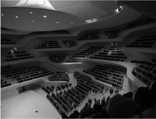
Figure 3: Acoustic model (1:10 scale) of the Elbphilharmonie in Hamburg by Herzog & de Meuron, 2016. Nagata Acoustics. (Plate 4, p. 290)
