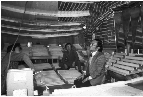
Figure 1: The first acoustic model used by Yasuhisa Toyota for the Suntory Hall project, Tokyo, 1986. Nagata Acoustics. (Plate 3, p. 290)
