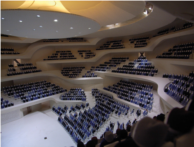
Plate 4: Acoustic model (1:10 scale) of the Elbphilharmonie in Hamburg by Herzog & de Meuron, 2016. Nagata Acoustics. (Figure 3, p. 125)
