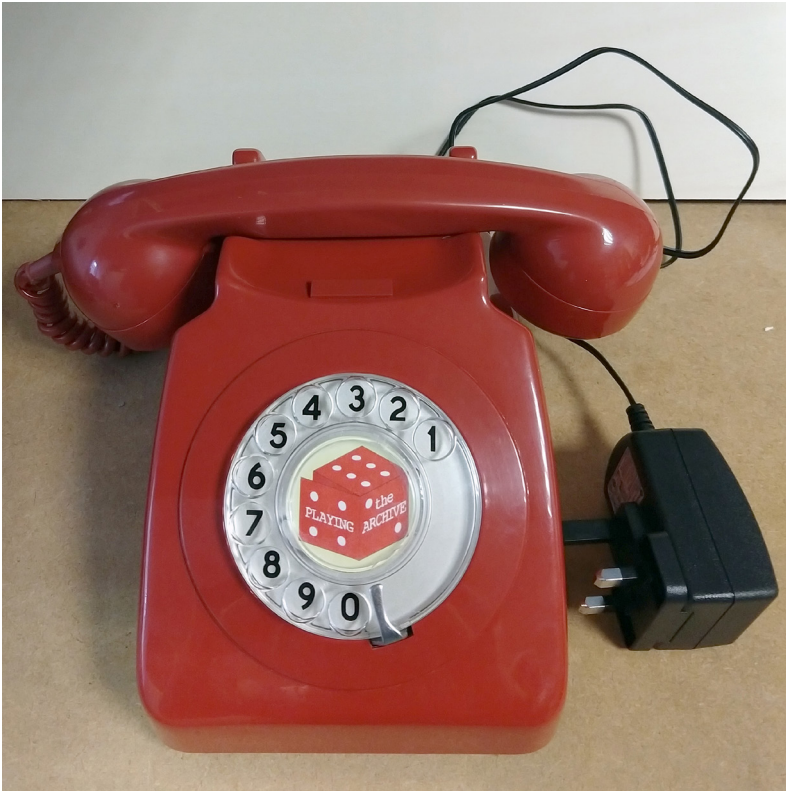
Figure 7.1 The first version of the retrofitted GPO 746 red rotary phone used as part of the Time Telephone installation at the Young V&A. © Valerio Signorelli.
