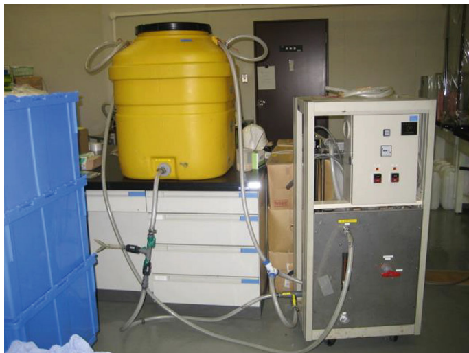
Fig. 14.2 Photo of the apparatus used for sterilization. The right-hand device is the water flow sterilizer (UVC-WSGL-10L, KURIKOU, Japan). The yellow tank is a 200 L polyethylene tank
