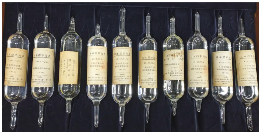
Fig. 11.1 A photograph of JSSWs stored at the JMA. From left to right, calibration year (chlornity) is 1950 (19.390‰), 1950 (19.394‰), 1948 (19.410‰), 1956 (19.387‰), 1951 (19.349‰), 1953 (19.372‰), 1943 [2603 in Japan's Imperial era] (19.39‰), 1956 (19.386‰), 1950 (19.395‰), and 1951 (19.355‰). All ampoules state that they were calibrated by the JSSWC, except for the 1948 ampoule, which states that it was calibrated by the CMO. Unlike SSW, which is sealed in ampoules made of soda glass, JSSW is sealed in borosilicate glass ampoules, and hence there are few suspended particles resembling glass flakes and crystals on the inner walls of the borosilicate glass
