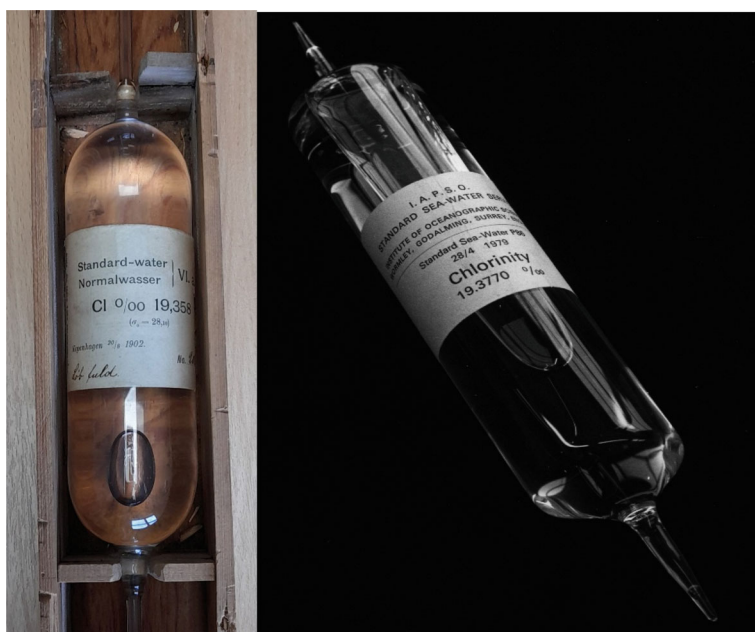
Fig. 8.2 Ampoules of Standard Seawater No. VIa (left) and P86 (right)
