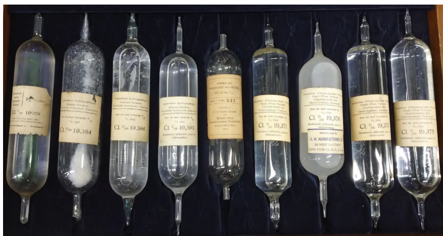
Fig. 11.2 A photograph of the historical SSWs and ASSW stored with the JSSWs shown in Fig. 11.1 at the JMA. From left to right, batch numbers (chlornity, calibration date) are P8 (19.379‰, 15 April 1913), P13 (19.384‰, 28 June 1929) (broken ampoule without seawater), P14 (19.386‰, 21 September 1932), P15 (19.393‰, 20 June 1937), ASSW batch 1 tube 537 (19.380‰, 1941) (used ampoule without seawater), P19 (19.371‰, 6 April 1950), P18 (19.376‰, 4 December 1949) (distributed by G. M. Manufacturing Co., N.Y., U.S.A.), P19 (19.371‰, 6 April 1950), and P21 (19.375‰, 29 March 1953). The ampoule of P18 contained white suspended material, as noted by Park (1964)
