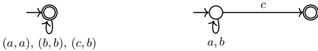
Fig. 3. Left: A transducer \mathcal{T} that converts each occurrence of letter c into letter b . Right: A weakly acyclic DFA \mathcal{A} accepting language (a+b)^*c .
