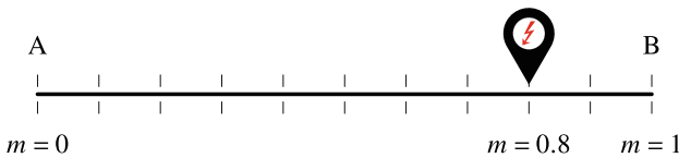
Fig. 10.25 Result of the fault localization of the MBP algorithm after a single-phase-to-ground fault in phase 1 with a relative fault distance of m = 0.8 at t = 0.1 s
