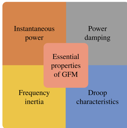
Fig. 2.5 Essential properties of grid-forming (GFM) VSCs inside a 100% inverter-based power system (IBPS)
