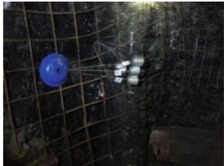
( b ) Multi-point Displacement Meter
