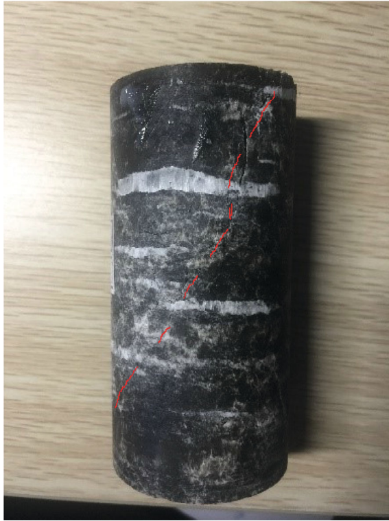
Fig. 3.19 Uniaxial compression test result of the specimen
