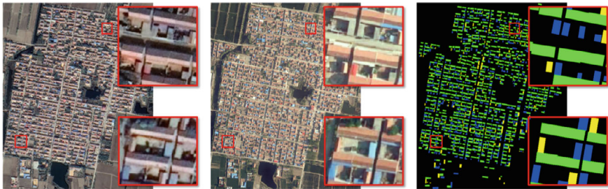
Fig. 5.3 Two types of open-source remote sensing satellite images and the actual labels for the corresponding roofs
