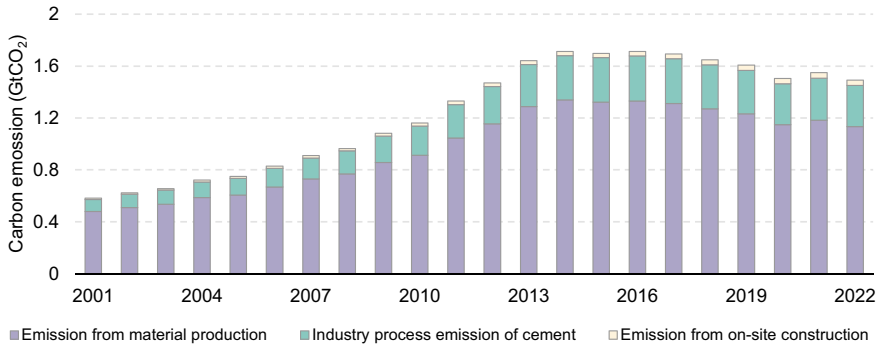
Fig. 1.14 Embodied carbon emissions of civil buildings in China (2004–2022). Source Estimation by BEREC, Tsinghua University. Note Civil building construction is included only
