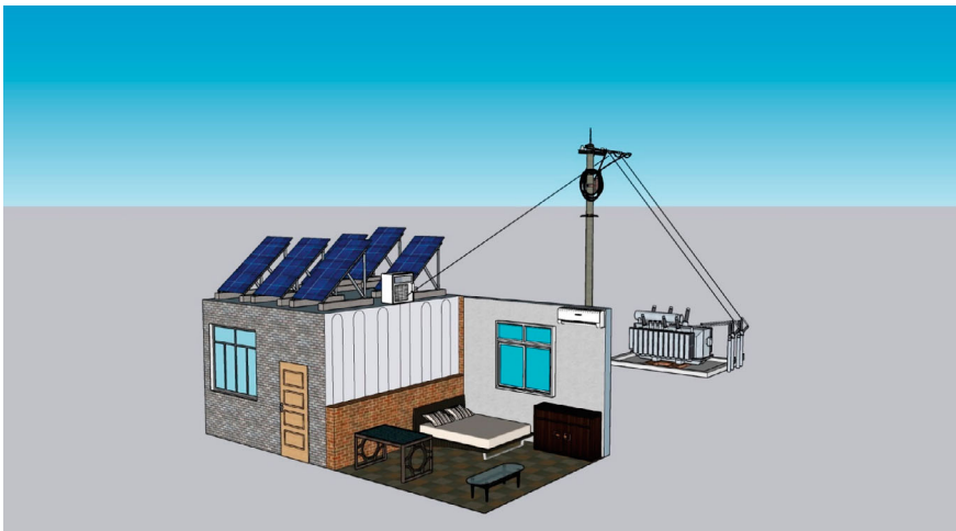
Fig. 7.4 Schematic diagram of PV heating system based on wall heat storage
