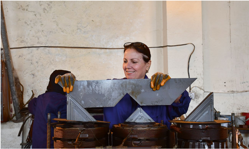
Naxşin Mohammed Amîn is a veteran technician and master at the Silêmanî Transformer Workshop. She is connecting transformer coils. By Sara Namo, Silêmanî 2022, Başûr. All rights reserved. The material is copyright protected and not governed by the same CC license as the rest of the work being published by Springer Nature
