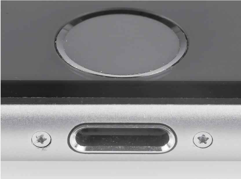
FIGURE 8.1 iPhone 6s pentalobe screws, lightning connector (proprietary) port and home button with Touch ID (proprietary).
