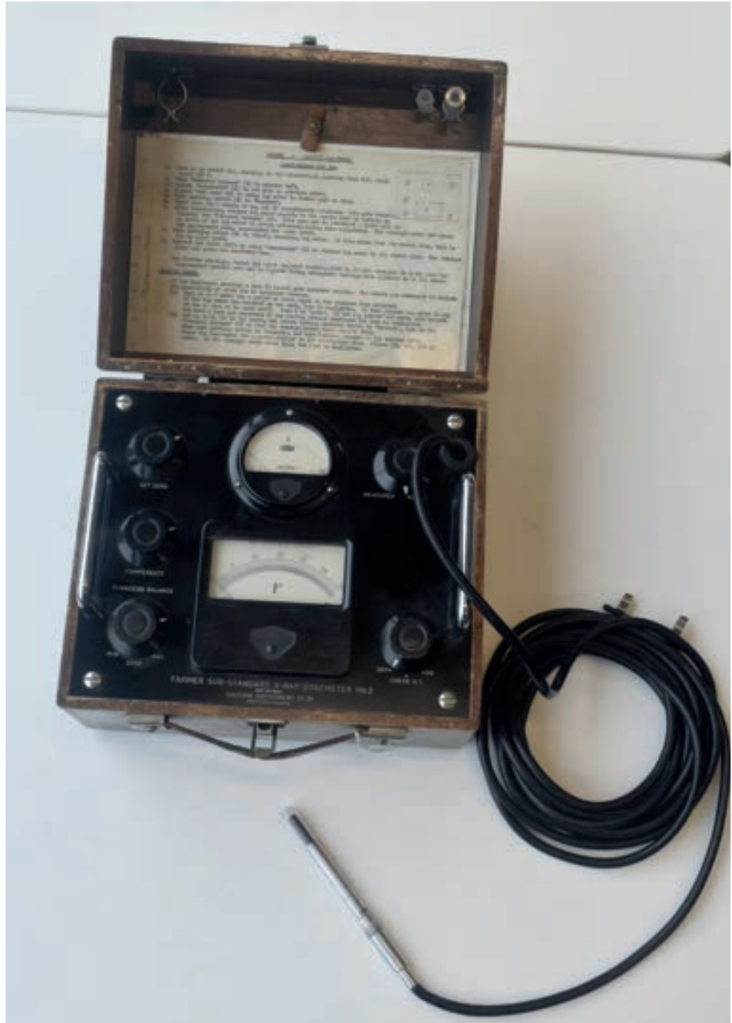
An early Baldwin-Farmer ion chamber connected to a high-sensitivity electrometer.
