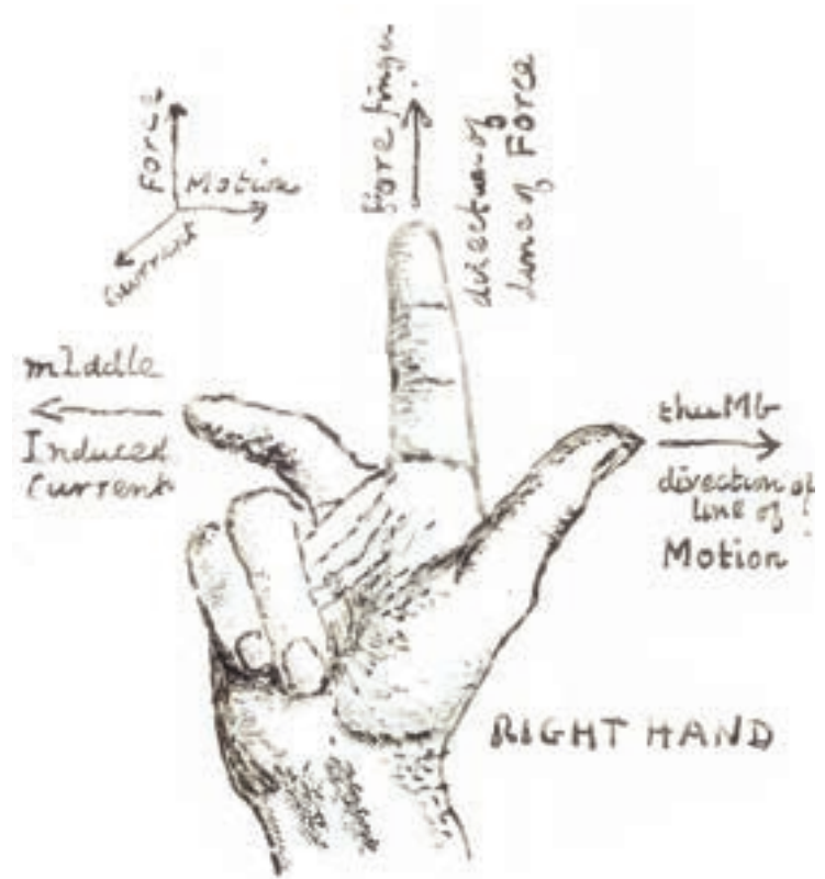
Fleming's right-hand rule, depicted on a glass slide used in teaching and probably drawn by Fleming himself.
