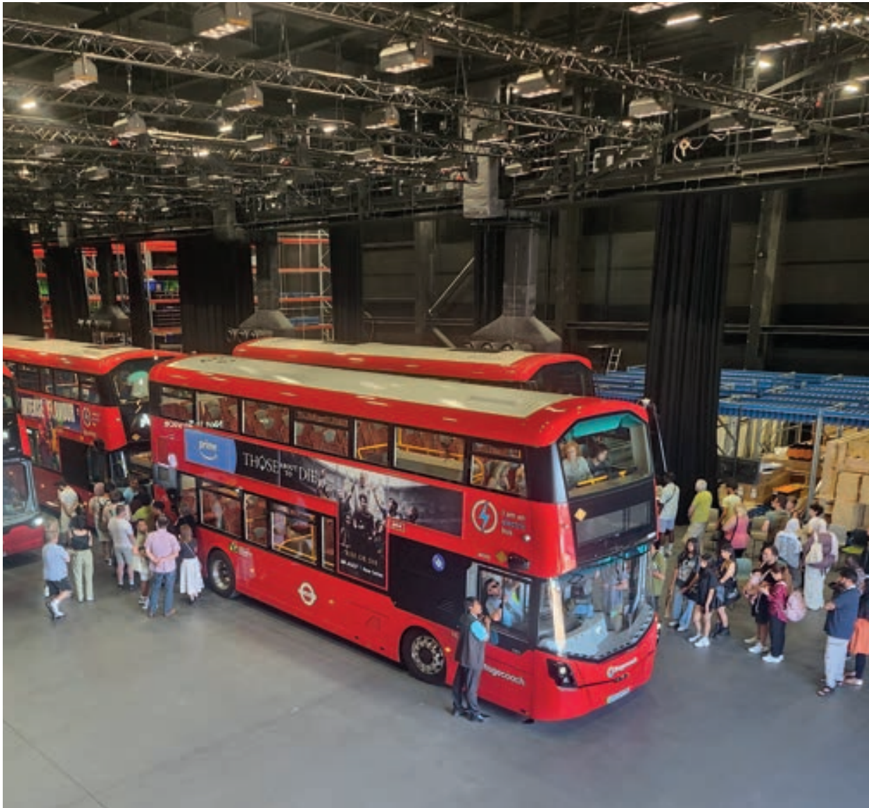
Four London double-decker buses inside PEARL during an experiment for Transport for London related to passenger responses on thermal comfort in buses.
