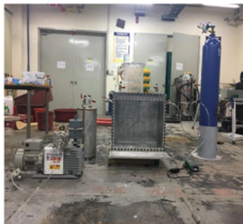
Fig. 16.5 Saturation system. (a) Schematic of saturation system (b) Actual saturation system
