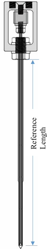
Fig. 1.11 Images of a new design for LEAP-2017 CPT device and rod lengths of the devices used at different facilities
