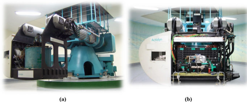
Fig. 16.1 Dynamic geotechnical centrifuge facility at KAIST centrifuge testing center: (a) centrifuge main body, (b) earthquake simulator
