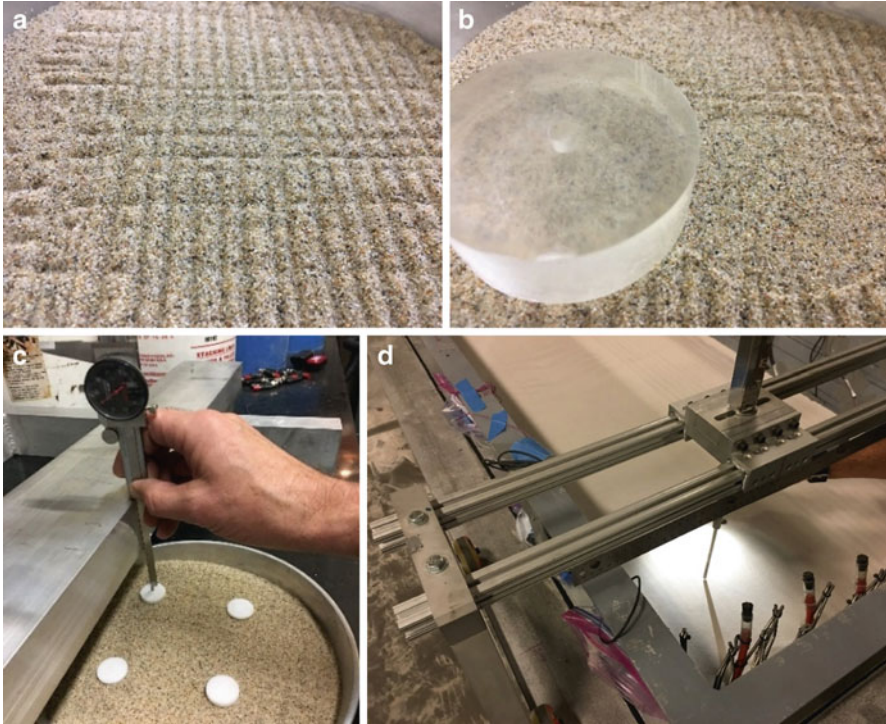
Fig. 1.4 Illustration of recommended method to measure the volume of sand specimen. (a) Rough surface of sand after shaping with vacuum. (b) 25 \times 70 mm acrylic disk lightly set down on surface, slightly twisted as necessary to smooth the surface. (c) 5-mm-thick \times 18-mm-diameter PVC or HDPE plastic disks gently placed on the smoothed sand in a grid. X, Y, and Z coordinates of the disk to be measured using caliper. (d) Measuring rails used on the large centrifuge at UCD. Good quality of light with a distinct shadow aids in resolving the location of the surface
