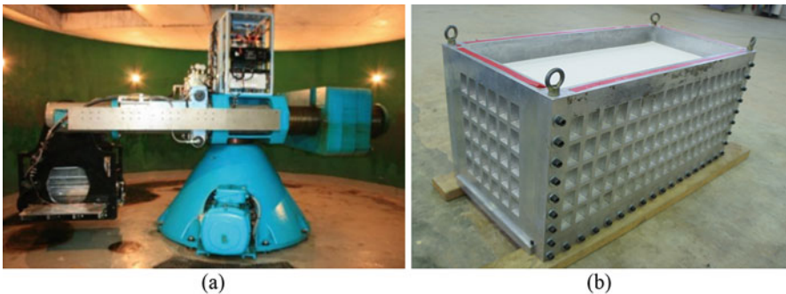
Fig. 18.1 (a) Geotechnical centrifuge at NCU (b) Rigid container
