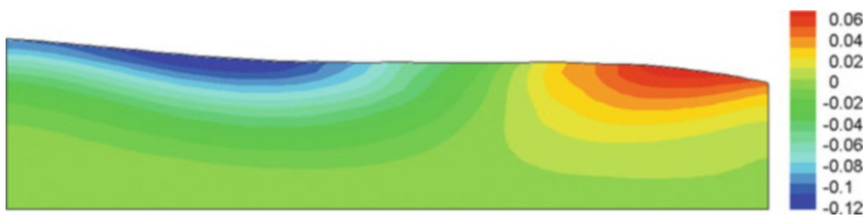
Fig. 29.13 Final vertical displacement contour (deformation of the model is amplified by 4 times, unit: m)
