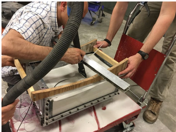
Fig. 13.2 Wooden template and vacuum tool used to excavate sand to produce the log-spiral surface
