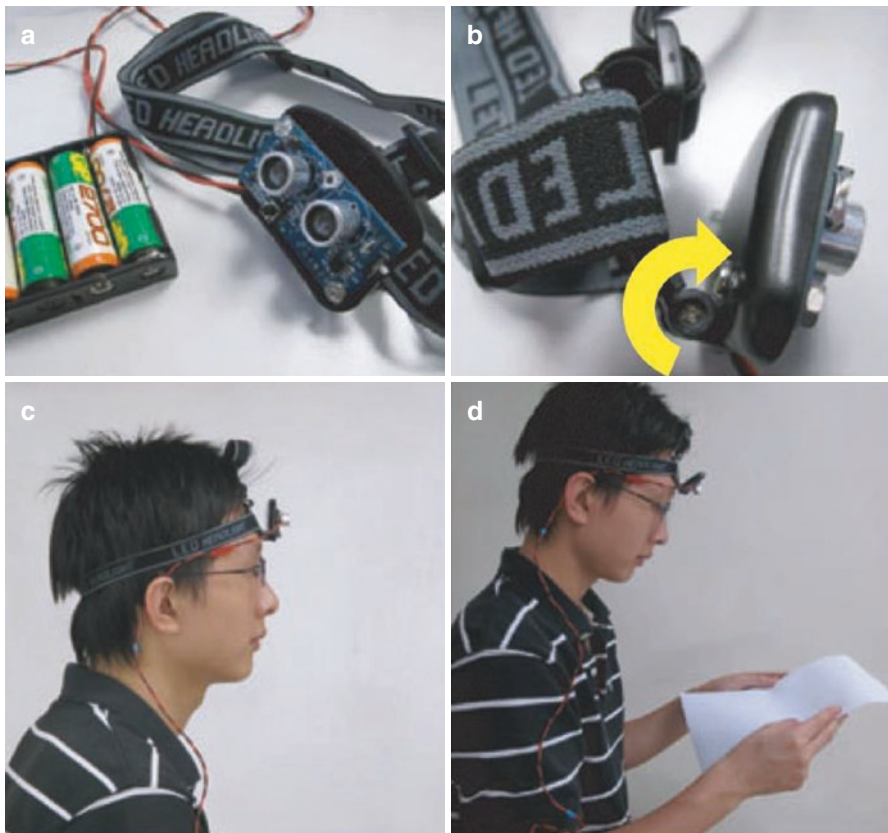
Fig. 7.7 Front view (a) and side view (b) of the near work analyzer for logging near work distance and its alignment in a straight-ahead position (c) and reading position (d). © Leung et al. [57]
