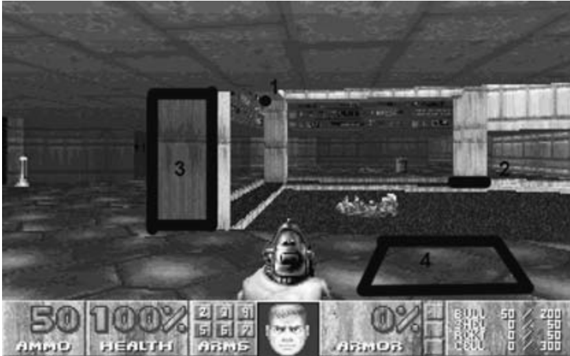
Fig 7. A vertex (1), linedef (2), sidedef (3), and part of a visplane (4) in DOOM's E1M1
