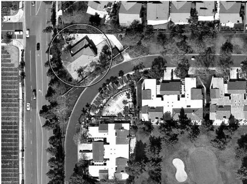
Figure 8.4 Extraction type satellite systems used to provide water to nearby golf course. Note: treatment plant (circled) looks like a residence, albeit a bit larger. The system has been in operation for more than 25 years.
