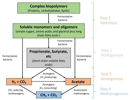
**Figure 1.1** Schematic representation of the anaerobic degradation of organic matter AD divided in four steps: (1) hydrolysis, (2) acidogenesis, (3) acetogenesis, and (4) methanogenesis.
