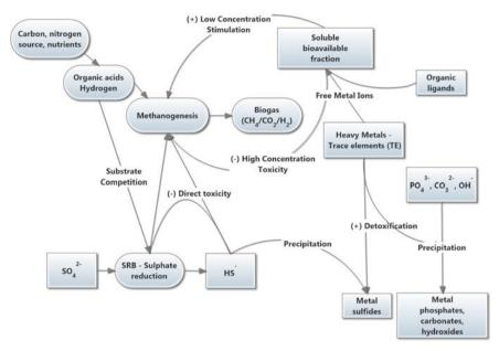
**Figure 5.2** Conceptual interactions between methanogenic activity, sulfate reduction and trace elements positive (+) or negative (-) effects on biogas production.
