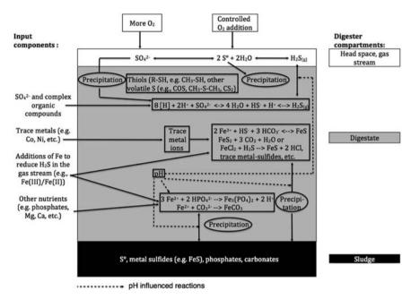
**Figure 2.2** Sulfur turnover in biogas bioreactors and its influence on TE and nutrients speciation (modified from Möller and Müller (2012) and reprint from van Hullebusch *et al.*, 2016).
