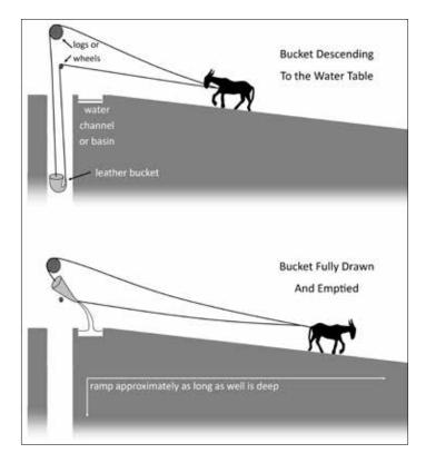
**Figure 1.5.** Cross-section of a *jalib*, or draw well
