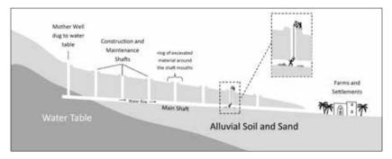
Figure 1.4. Cross-section of a qanat, or "chain of wells" Source: Lightfoot, "Origin and Diffusion."
