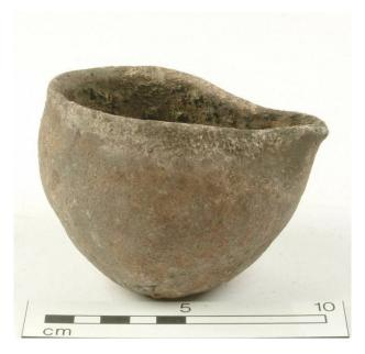
Figure 4. Saxo-Norman Crucible, mid-11th to mid-12th century, ceramic; earthenware, H 78 mm; DM (rim) 103 mm. Museum of London #13175.
