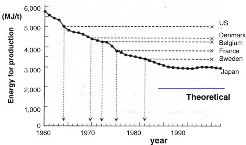
Fig. 4 Energy consumption for cement production. Source: Japan Cement Association
