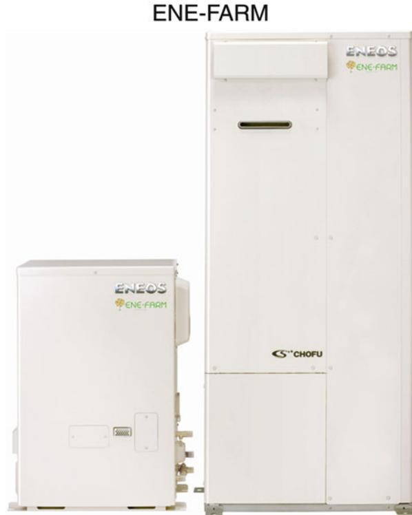
SOFC-type fuel cell was placed on the market in Japan. It achieved an impressive power generation efficiency of 45 %, and an overall efficiency of almost 90 % (since 42 % of the thermal energy emitted is used to produce hot water) (JX Nippon Oil & Energy Web-Site 2013).
