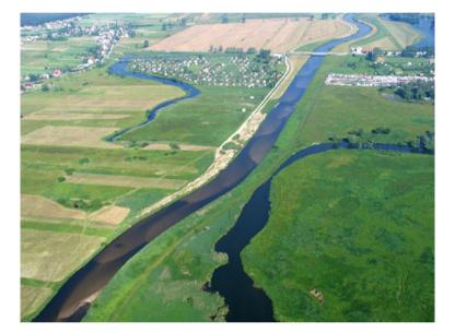
Fig. 5.3 Bedforms squeezed in a regulated channel (Source Pińczów Aero-club)
