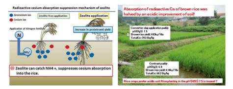
**Fig. 2.13** Technology to inhibit absorption of radioactive cesium (*left*), and the technology under trial (*right*) (From soil fertilization team data provided)
