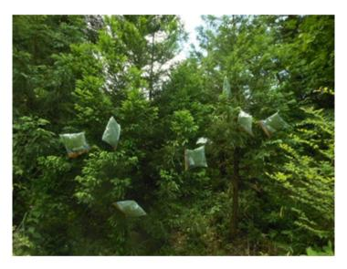
Fig. 13.5 Trapping transpiration water from the leaves of young *Cryptomeria japonica* using plastic bags in June 2013
