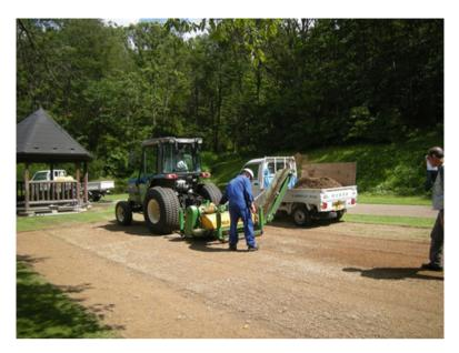
Fig. 11.1 Practical experiment using a field top maker to decontaminate a park lawn area
