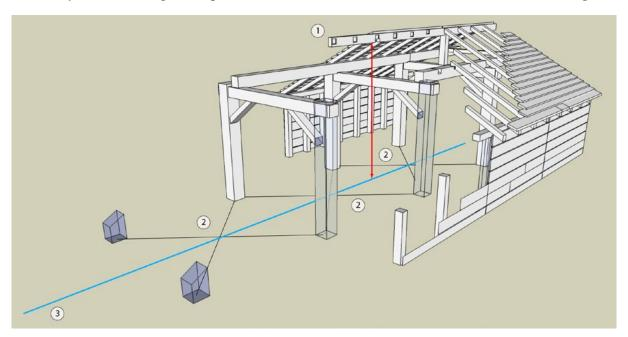
**Figure 6.** Three dimensional representation of the geometric principle. The main axis line (3) coincides with the uppermost part of the roof (1). The roof supporting pairs are located in diagonal relation to this line (2).
