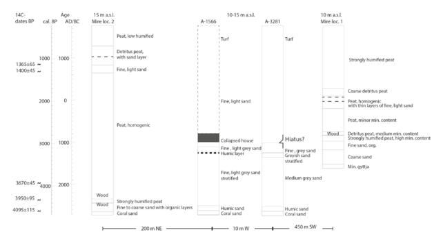
Figure 12. Correlation of sediment profiles from Sandvika. The main chronology is based on Bayesian radiocarbon calibration (Buck et al. 1999) and a linear age-depth model (Bennett 2005). The chronological placement of the stratigraphic layers of A-1566 (except Collapsed house) and A-3281 is tentative.
