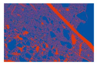
Fig. 198: Coarse plaster under the ESEM microscope, grains coloured blue, pores coloured red.
