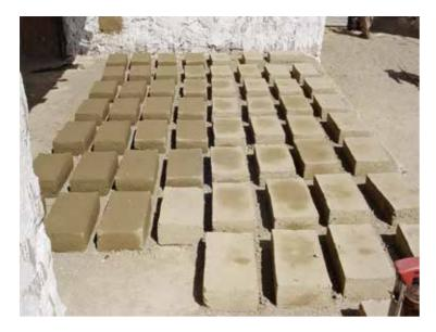
Fig. 56: Adobe mud bricks used for historical and conversation wall construction in the Western Himalayas.
