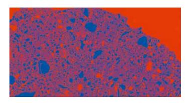
Fig. 199: Fine plaster under the ESEM microscope, grains coloured blue, pores coloured red.
