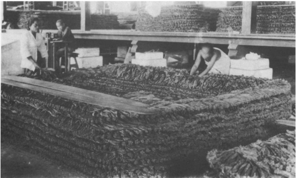
29. Graded tobacco bundles are placed in large piles for the fermenting process. Long bamboo tubes reach to the center of the tobacco piles and permit the measuring of the temperature in the interior of the piles. Before the temperature reaches dangerous levels the piles are rearranged. Deli, East Sumatra. (DPV)
