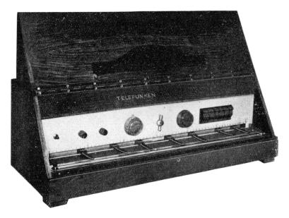
**FIGURE 23.** The Telefunken-Trautonium, also known as the Volkstrautonium. Source: Peter Lertes, *Elektrische Musik* (Dresden: Theodor Steinkopff, 1933), 184.
