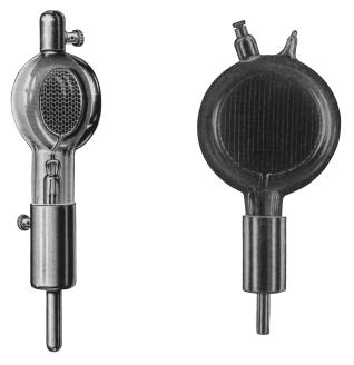
**FIGURE 14.** Photoelectric cells. These tiny devices transduce light into electricity; they were central to the development of optical sound film. Source: Heinrich Geffcken, Hans Richter, and Joachim Winckelmann, *Die lichtempfindliche Zelle als technisches Steuergerät* (Berlin: Deutsch-Literarisches Institut J. Schneider, 1933), 37.
