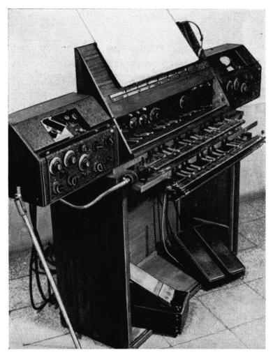
**FIGURE 25.** The three-voice Trautonium, circa 1936. To the original monophonic sound module (center), two additional modules have been added. Three playing manuals are located below the center module. The pedals on the right control volume; the one on the left allows for continuous modification of tone color. Source: Friedrich Trautwein, "Wesen und Ziele der Elektromusik," *Zeitschrift für Musik* 103, no. 6 (1936), unpaginated photo insert.
