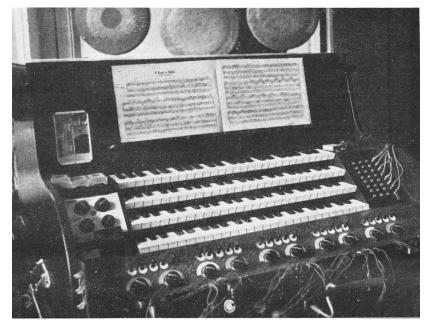
**FIGURE 26.** The five-voice Partiturophon, circa 1934. Both Mager's and Trautwein's instruments continued to grow during the 1930s, but both achieved polyphony only by multiplying monophonic manuals. Source: "Das 'Partiturophon'—Eine Hausmusik-Lösung," *Zeitschrift für Instrumentenbau* 54, no. 21 (1934): 329.
