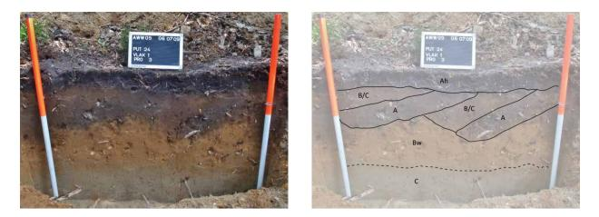
Fig. 5.11: Profile 24.3. Example of completely ploughed soil profile.
