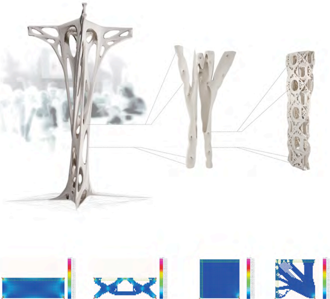
Picture 2: Evolutionary Plasticity – concept models and example diagrams illustrating the removal of low stress regions using Evolutionary Structural Optimization (Xie & Steven)
