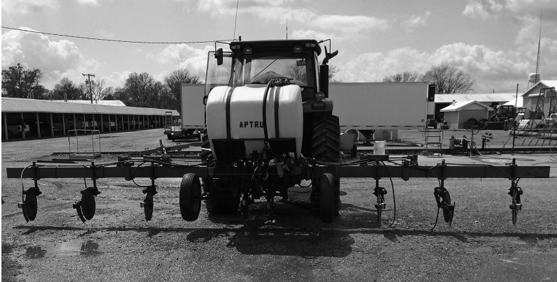
FIGURE 6.1 A map-based variable-rate liquid fertilizer applicator. Prescription maps can be uploaded and displayed in the controller installed inside the cab.
