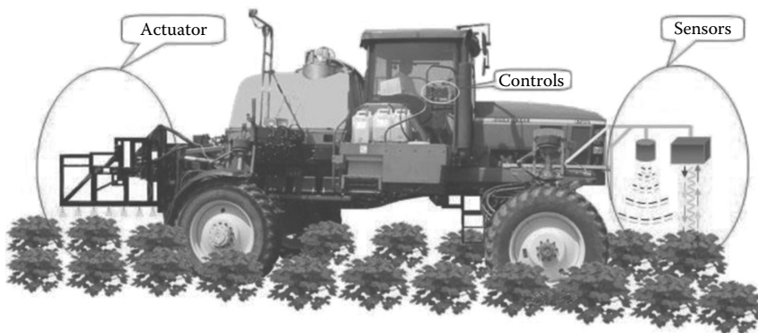
FIGURE 6.2 Illustration of a sensor-based variable-rate application system including sensors, controls, and the actuator.
