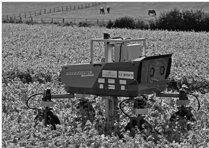
FIGURE 5.17 BoniRob autonomous field robot with a soil penetrometer application module. (From University of Applied Sciences Osnabrück, Germany. With permission.)
