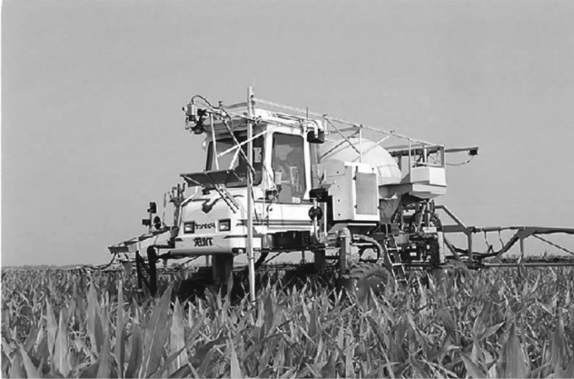
FIGURE 4.13 An example of an intelligent variable-rate applicator. The machine-mount crop sensing system is capable of self-calibrating to natural lighting conditions.
