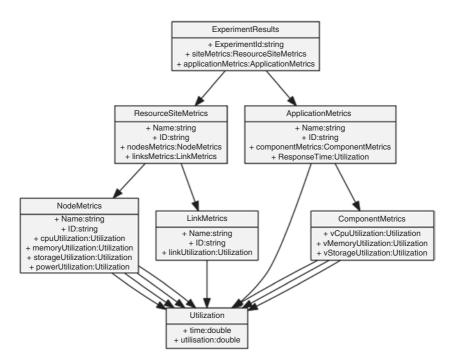
Fig. 5.3 DES simulation results format (outputs)
