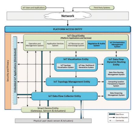
Fig. 6.13 SAT-IoT platform architectural model
