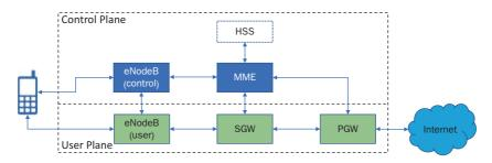
Fig. 6.2 A forwarding graph of a network service in an LTE network
