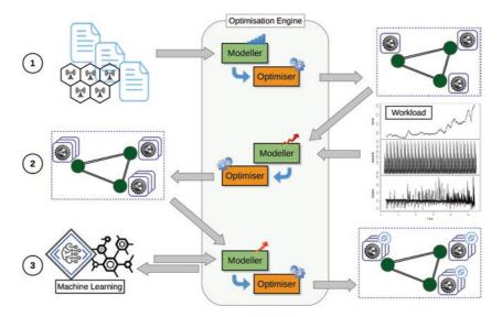
**Fig. 3.1** A stratified approach to application optimisation iteratively building on three optimisation building blocks—(1) classic optimisation on static data, (2) application adaptation to variations in workloads and resource availability, (3) joint autoscaling and optimisation in multi-tenancy scenarios using machine learning (adapted from Le Duc et al. (2019))
