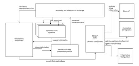
Fig. 1.3 Component-oriented overview of the RECAP optimisation subsystem
