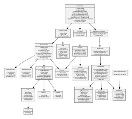
Fig. 5.2 DES simulation model data format (inputs)
