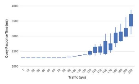
Fig. 6.23 LKN system performance under different traffic scenarios
