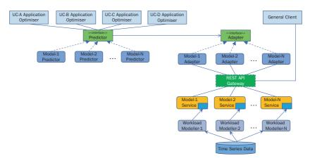
Fig. 3.2 A platform for the integration of predictors and modellers
