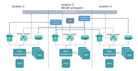
Fig. 2.3 RECAP's distributed monitoring architecture
