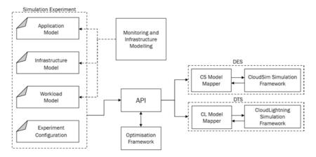
Fig. 1.4 High-level overview on RECAP simulation framework
