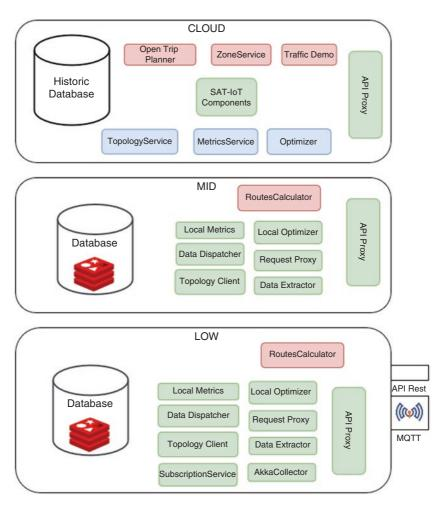
Fig. 6.14 SAT IoT platform high-level conceptual architecture
