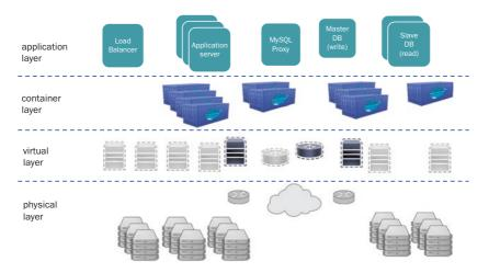
Fig. 2.2 RECAP monitoring layers
