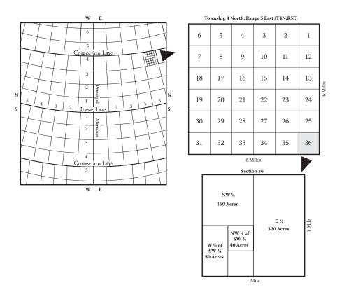
*Figure 2.1* The US Rectangular Survey System (redrawn from Johnson, H., *Order upon the Land*, Oxford, 1976). Thus, the location of the NW quarter of the one square mile unit at the lower right of the diagram (termed a "section") would be northwest quarter of Section 36, Township 4 North, Range 5 East, abbreviated NW ¼, Sec. 36, T4N, R5E. In the Hill Country, tracts as small as 40 acres (16 ha) could be purchased, and tracts were not always contiguous.
