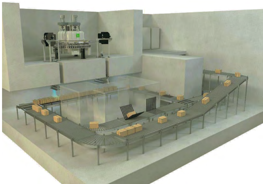
Figure 3. Electron beam irradiation facility equipped with an electron accelerator and electron-to-X radiation converter. (Photo from Ion Beam Applications (iba), reproduced with permission.)
