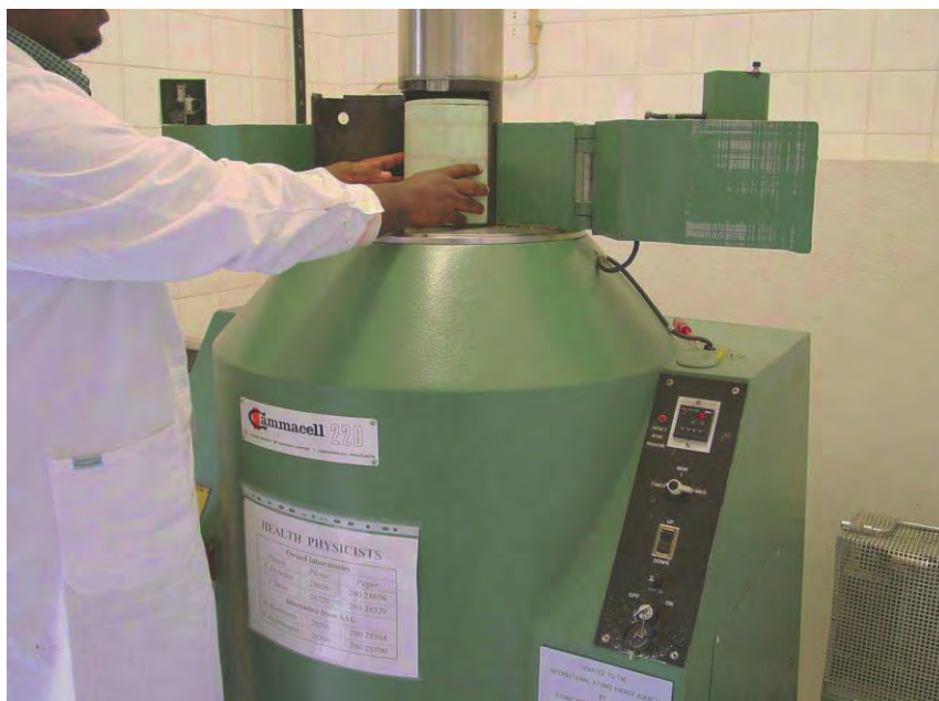
Figure 1. In preparation for irradiation, a canister with insects is placed in the irradiation chamber (while it is in the shielded position) of a self-contained gamma irradiator. Depending on the dose rate of the day, the timer on the control panel (lower right) is set to give the desired dose.
