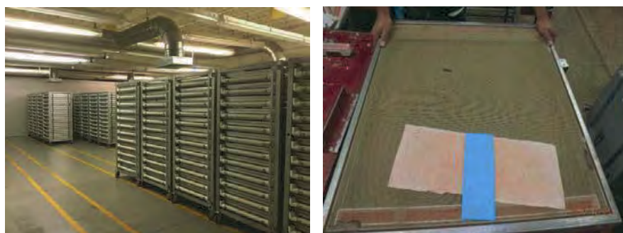
Figure 5: Left: Fly emergence and maturation room inside the new ERF at El Pino, Guatemala, using liquid-diet towers, with air-conditioning units for room conditioning. Right: Liquid-diet tray showing (through the screen) two white plastic trays holding pupae (pupae marked with orange-coloured dye). A cotton cloth (white) and a sponge (blue) draw the liquid diet by capillary action from the PVC-pipe system placed on the side of the trays (as shown in the left photo).
