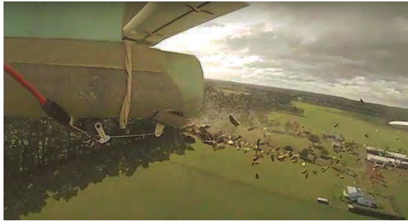
Figure 16. Remotely piloted fixed-wing drone, operated in visual line-of-sight, releasing sterile codling moths in New Zealand (PFR 2018a, b). (Photo from R. M. Horner and Plant and Food Research Institute, New Zealand (PFR 2018a), reproduced with permission.)
