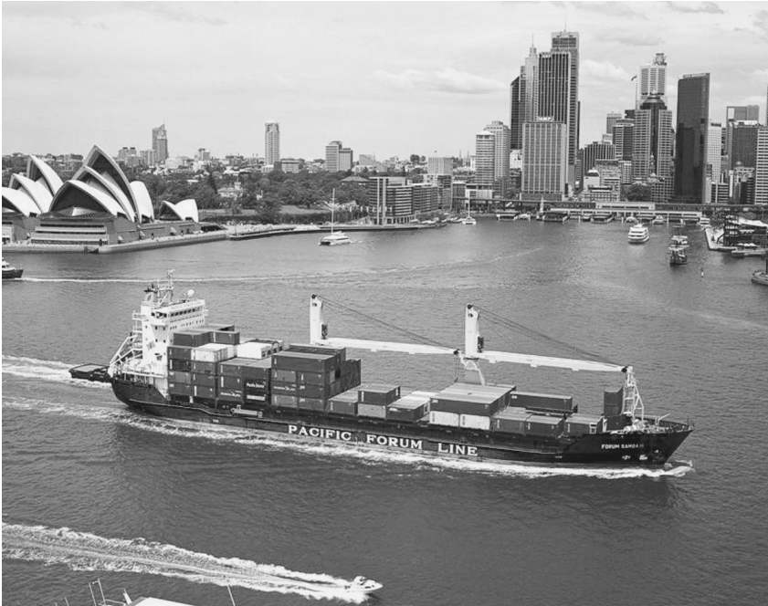
FIGURE 10.4. The Pacific Forum Line's Forum Samoa II (2002)—like her sister ship, Captain Tasman —carries 310 containers and has refrigerated and bulk liquid space, a twenty-six-ton gantry crane, a Ro-Ro ramp, and a speed of 15 knots. She has a crew of thirty, which includes a large number of trainees. (Courtesy of the Pacific Forum Line)
