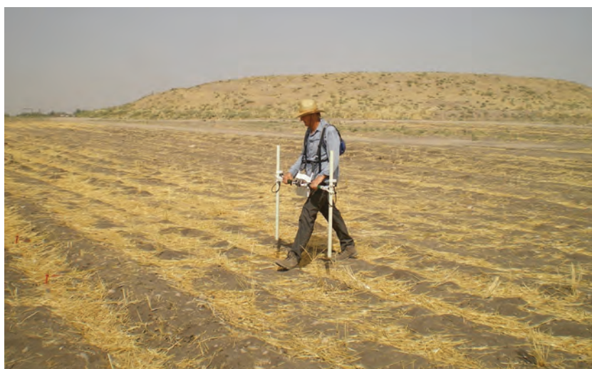
Figure 5.1. Fluxgate gradiometry survey over the area southeast of the mound.
