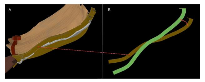
Figure 5. Slant view (A) of hull from stern at 30° vertical rotation showing twisted keelson and keel (red-brown), and end view (B) of hogged ribs cracked 20°.
