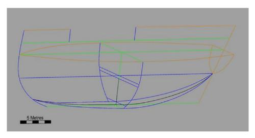
Figure 4. Reconstruction of the Santiago de Galicia ship, based on historical documents. Colours represent origin of sources. Green for direct evidence from documents, blue for estimated dimensions based on the overall basic dimensions in green, brown is indirect evidence of the time, collected from examples of ships specified in the Spanish Ordenanzas.
