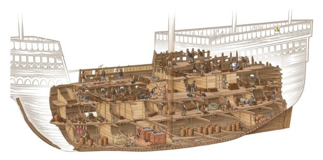
Figure 5. Isometric drawing of the hull with an interpretation of the men and objects (© Mary Rose Trust).
