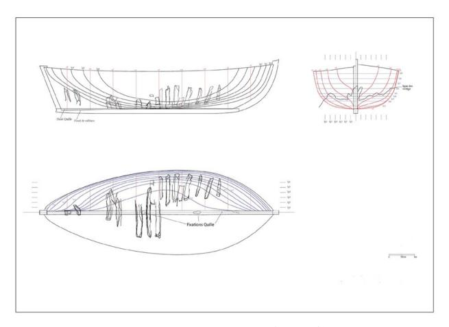
Figure 5. Reconstruction of the vessel lines (S. Bertoliatti).
