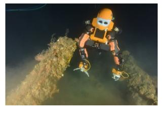
Figure 3. Trials of Techno-Concept's robotic hand off Toulon (F. Osada and T. Seguin, 2014 © DRASSM).
