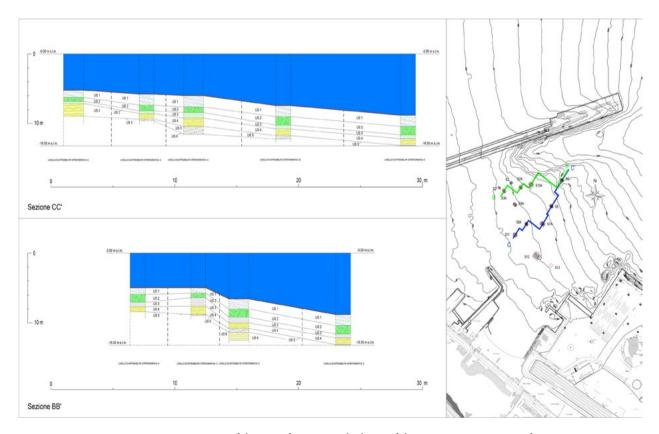
Figure 3. Reconstruction of the stratification on the basis of the sixteen surveys carried out.
