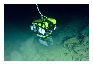
Figure 2. DRASSM'S ROV *Hilarion*, fitted with heavy sampling claws (F. Osada and T. Seguin, 2015 © DRASSM).
