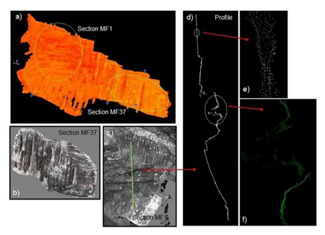
Figure 2. Intensity point cloud of the ship wreck at the museum (a), rendered 3D point clouds based on the underwater images captured of the *Batavia* – Section M37 (b) and section MF1 (c), selected profile of MF1 (d) and its detailed views 1 (e) and (f).
