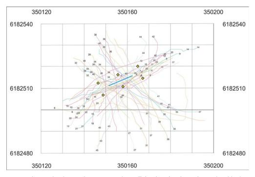
Figure 2. The 48 sailing lines at the experimental site off Skovshoved Harbour. The 12m long blue line marks the position of the linear string of samples placed on the seabed. The six yellow rectangles mark the buoys used to control the boat's approach to the target.
