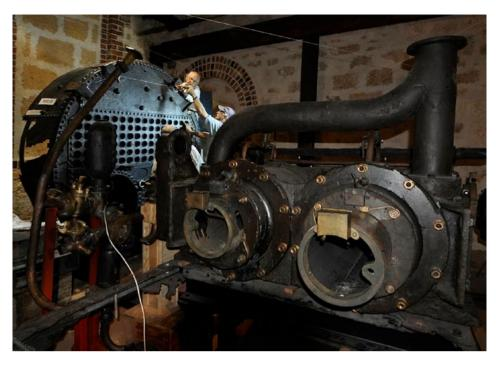
Figure 3. the Museum's Marine Engineers, with R. Garcia at work constructing the *Xantho* engine room. Foreground the engine and its piping (M. McCarthy, Western Australian Museum).
