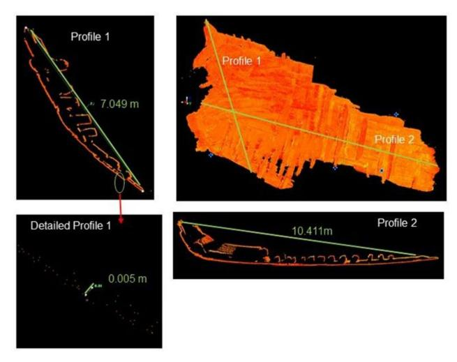
Figure 1. Point Cloud of the *Batavia* shipwreck captured with the Leica C10 laser scanner at the museum (top right) as well as two selected profiles (top left and bottom right) with a detailed section (bottom left).
