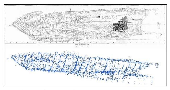
Figure 3. Henderson's 2D plan drawn from 1975–76 underwater survey of *James Matthews* site with 27 x 1m grid sections shown underneath (top), and oblique view of point cloud data used to create the *James Matthews* 3D digital model (below).
