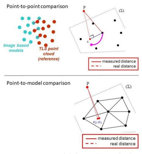
Figure 3. Point-to-point comparison (top) and point-to-model comparison (bottom) (adopted from CloudCompare, 2017.)
