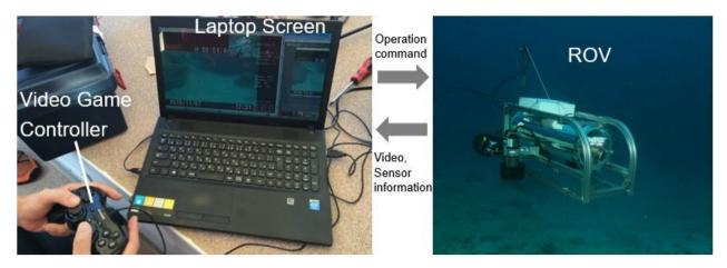
Figure 2. ROV and its operating system (Yuji Yamamoto).
