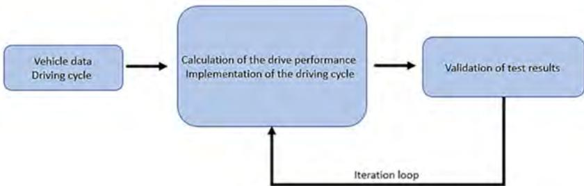
Figure 3.2: Research method Calculation of drive performance.
