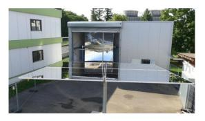
Figure 1: Solar furnace arrangement consisting of a heliostat mirror (front, outside) and a parabolic mirror (back, inside the laboratory) (Foto: J. Flesch).
