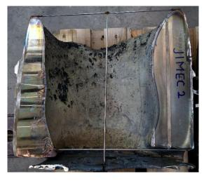
Figure 6: Cut of the test substrates of JIMEC-1 and JIMEC-2
