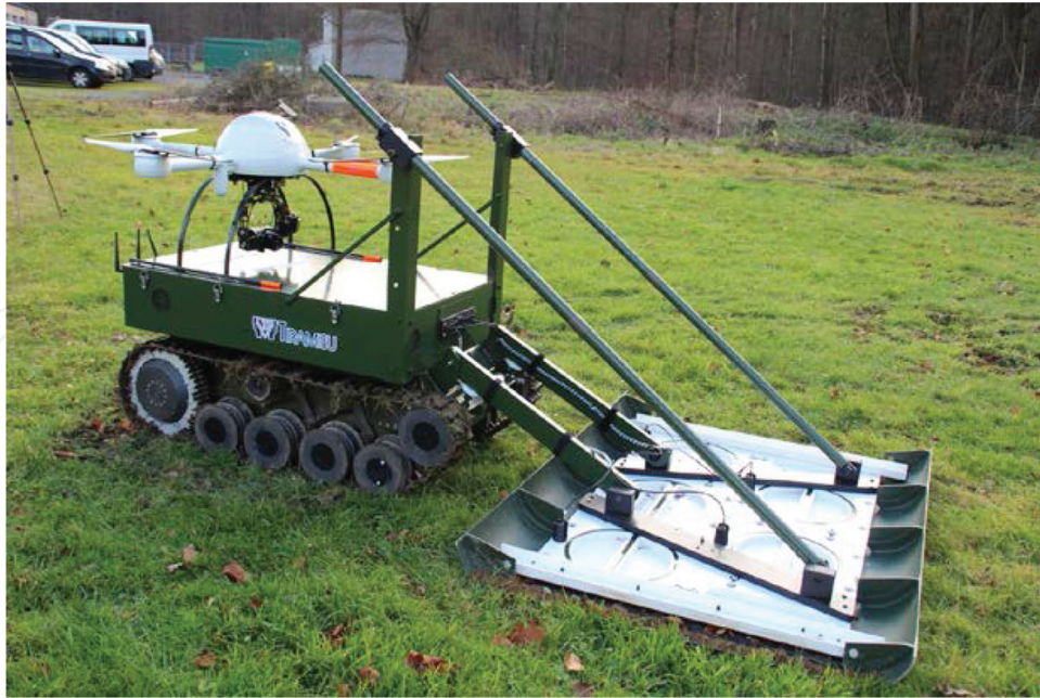
Figure 7. The teoDOR equipped with the MCMD and a TCP box positioning system.
