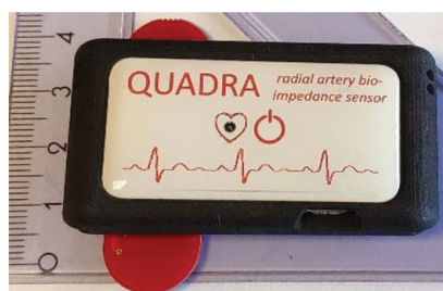
Figure 3. The prototyped version of a wearable impedance measurement device.
