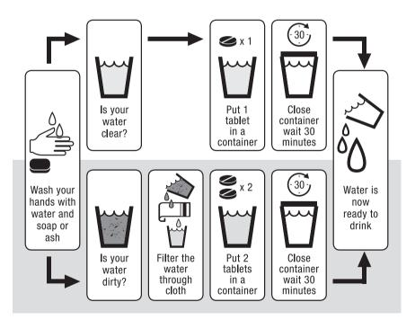
FIGURE 5.2 Water treatment using chlorine tablet
