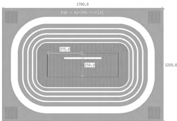
Figure A.4 Layout of an LGAD-LGAD pair in the TI-LGAD production (dimensions shown in \mu\text{m} ).
