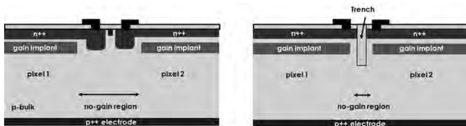
Figure 5.14 Comparison between the standard ( left ) and the trench-isolated ( right ) LGAD designs.
