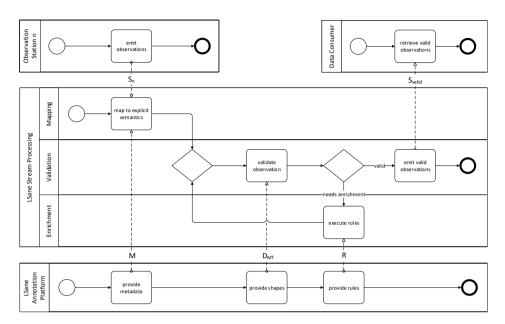
**Figure 4.2:** Overview of the system architecture of LSane: Ambiguous observation messages emitted by various observation stations are mapped to explicit semantics based on metadata M provided by a corporate knowledge graph, validated using the definitions of  $D_{MT}$ , and enriched if needed using rules of R. Finally, observations that conform to the shape constraints contained in  $D_{MT}$  are emitted for the data consumer.
