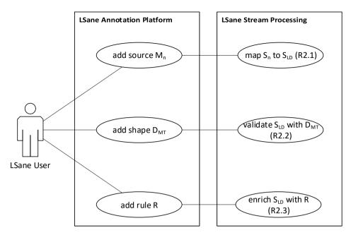
**Figure 4.6:** Use cases of LSane: adding metadata  $M_n$  triggers LSane to subscribe stream  $S_n$  and maps each message to  $S_{LD}$  (R2.1). Adding a shape constraint to  $D_{MT}$  triggers LSane to validate each message in  $S_{LD}$  using  $D_{MT}$  (R2.2). Adding a rule R triggers LSane to enrich each message in  $S_{LD}$  using R (R2.3).
