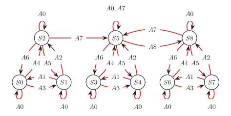
Figure 5.2: Effect (T) of actions A0 to A8 applied to states S0 to S8
