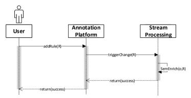
**Figure 4.9:** Provide rules R for further enrichment of sensor observation messages in  $S_{LD}$ .
