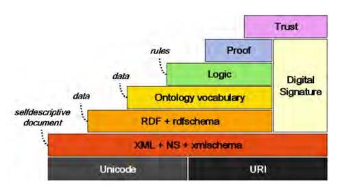
**Figure 2.3:** Layers of the semantic web technology stack [Koivunen and Miller 2001]: Ontologies are built on top of RDF that supports logic for proofing statements. Trust can be implemented on top of proofs and digital signatures.
