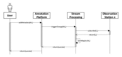
**Figure 4.7:** Register new stream  $S_n$  of sensor observations by providing metadata  $M_n$ .
