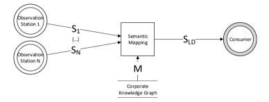
**Figure 4.3:** Overview of semantic mapping process: Each message without explicit semantics in each data stream  $S_n$  of heterogeneous observation stations is mapped to a new stream  $S_{LD}$  with explicit semantics based on metadata M of the corporate knowledge graph.
