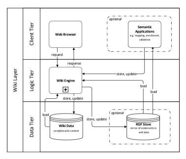
**Figure 3.1:** Architecture of SMW (own illustration based on [Krötzsch et al. 2006]): the wiki layer covers all aspects of both, semantic data management and also user friendly representation of the resulting corporate knowledge graph by including unstructured content and wiki markup. Although semantic applications may read data from an optional RDF store that mirrors statements of the wiki, updates still have to be performed using the wiki engine as the single source of data authority.
