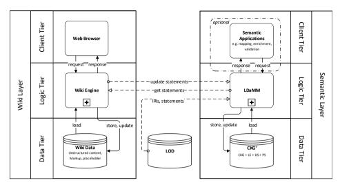
**Figure 3.2:** Architecture of the LD-Wiki-approach: wiki layer for a user friendly representation of the corporate knowledge graph by including unstructured content and wiki markup, semantic layer for enriching the corporate knowledge graph with Linked Open Data and curating it.
