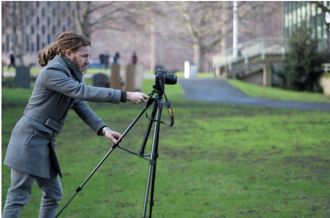
Figs. 52–53 The tripod dolly: the tripod's front legs remain stationary as the entire set up is pushed forward. The tripod's head is loosened so that the camera can remain perpendicular to the ground.
